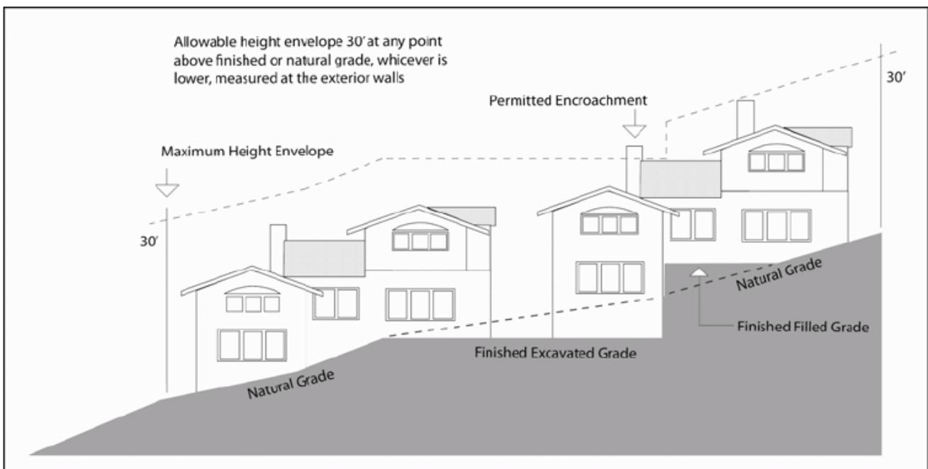
Figure 3-2. Height Measurement
